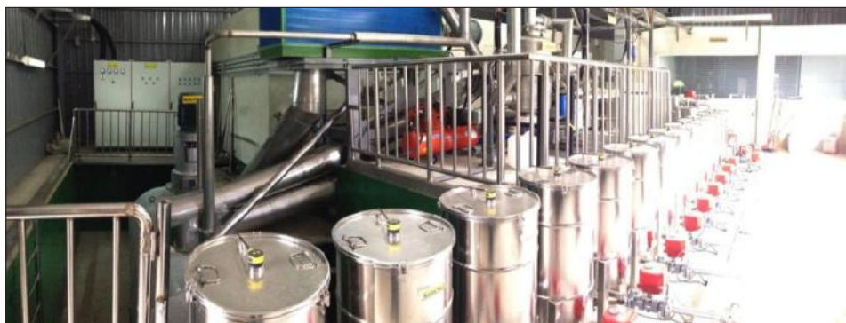
Figure 6: Photograph of first pilot facility for supertorrefaction of biomass into biocoal built by the HX Team on a site of the National Tsing Hua University in Hsinchu, Taiwan.
