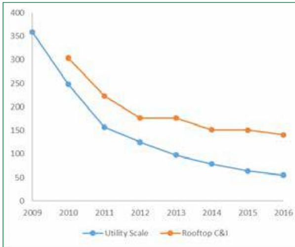
Figure 17: LCOE for solar PV in South Africa, 2009 to 2016 for utility scale and for commercial and industrial (C&I) rooftop installations, in US$ per MWh
